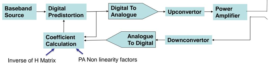
The DPD shall be designed as FPGA with dynamic look up table or with a fast DSP.
