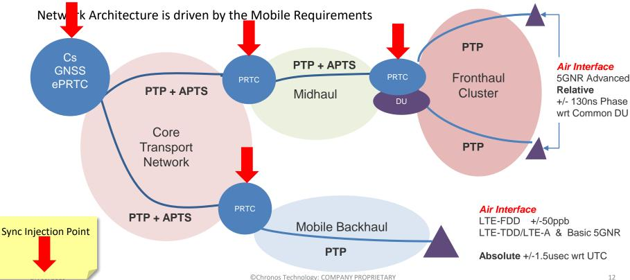
5GNR: Advanced Carrier Aggregation Services, wideband to the UE requires stringent TAE control to mitigate CoChan Interference
