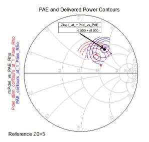
Load for optimum **PAE** at 1dB Compression for 8x50µm device biased at 75mA/mm at 4V
