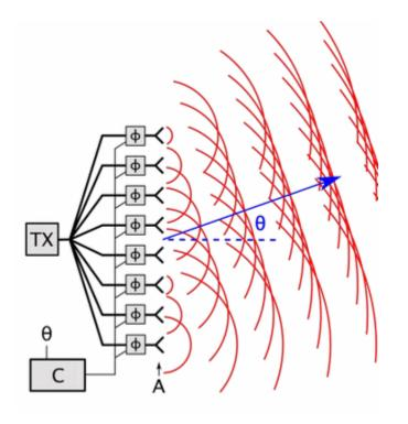
This is achieved by the additive/destructive effects of waves transmitted from multiple individual antenna elements controlled in phase and amplitude
