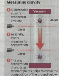
before you notice it. But by harnessing sophisticated quantum mechanical techniques, Professor Bongs, working with the National Physical Laboratory in southwest London, believes that they are close to developing their gravimeter into something portable that can spot tiny changes in density to "see' below the ground — all by observing the behaviour of individual atoms.
